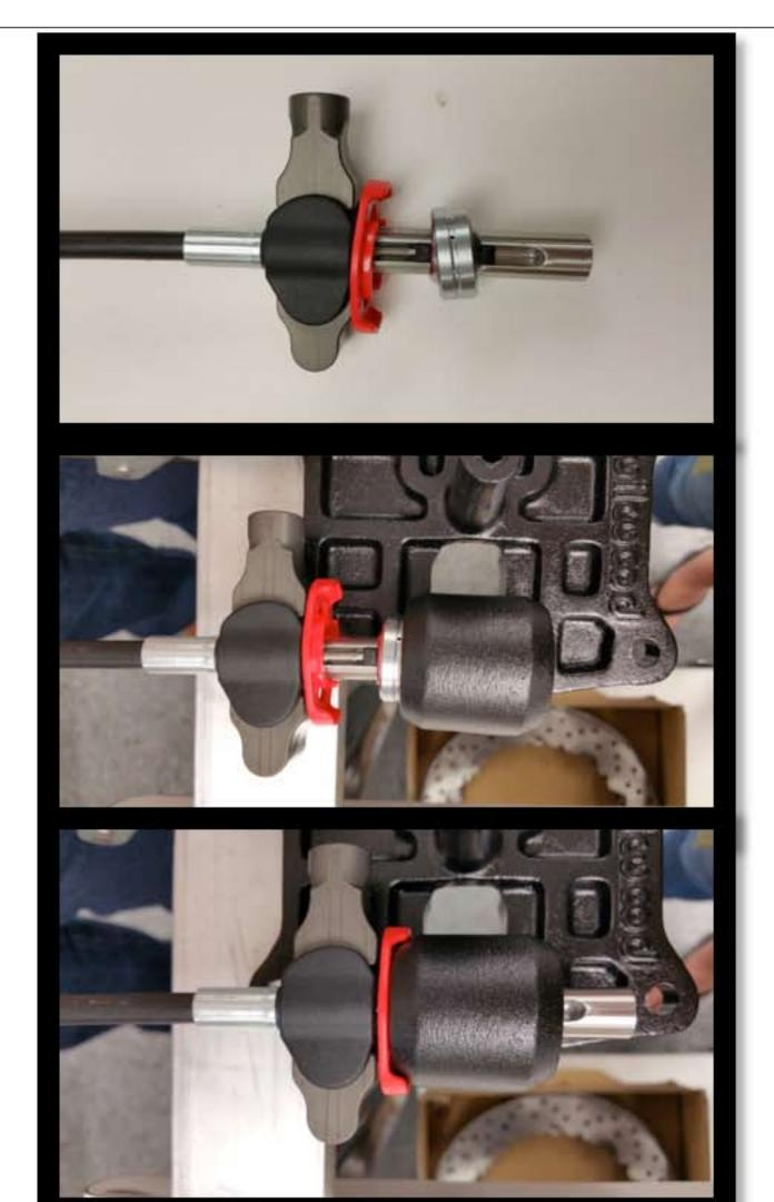
STEP 4 – Use supplied zip ties to secure red clevis guides to pedal, making sure that the flange on the clevis guide is installed as pictured. (Safety wire could be used instead of the zip ties, if preferred.)
