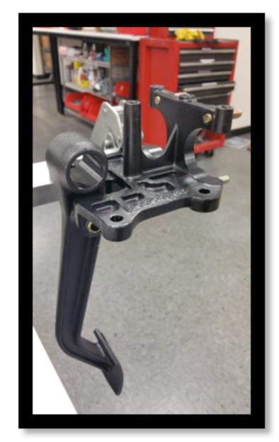
STEP 2 – On QTM bias shifter, remove clevis on the non-cable side of the assembly using allen wrench
