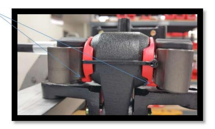
STEP 5 - Slide clevis onto bias shaft, making sure that it is timed correctly and re-install allen bolt through clevis into the bias shaft (use blue loctite).
