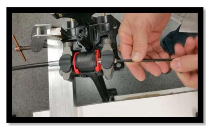
STEP 6 – Cycle cable back and forth by hand to ensure free movement of Rod-End Bearing at the pedal.
